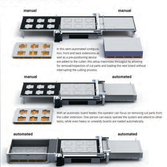
The highest level of automation includes automatic board feeding for loading, automatic stacking for off-loading. Manpower requirements are reduced to job setup, and delivery/removal of stacked boards. With this setup, it is possible to run the cutter without an operator in attendance.
