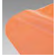
Balloon silk E.g. coated and rubberized fibers; man-made, waterproof materials.
