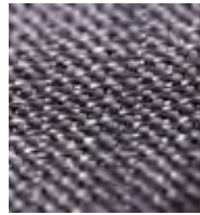
Carbon fiber in woven, non-woven, unidirectional form; single or multi-layer.
