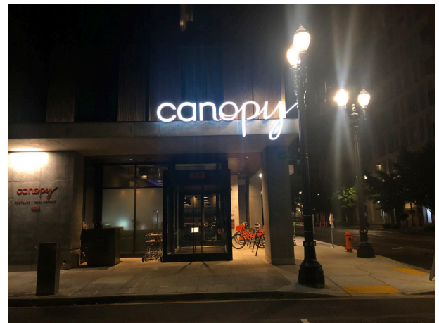
At night time, the internal lighting overwhelms the perforated film and changes the appearance to white or it takes on the color of the sign face used.
